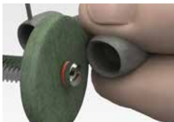
Shave off of the extended margin by using the rubber wheel.
