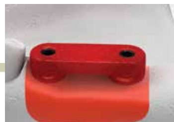
Fabricate the positioning jig
