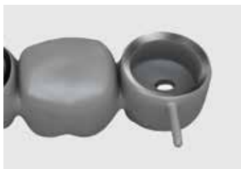
Metal framework after the removal of the "Lip".
